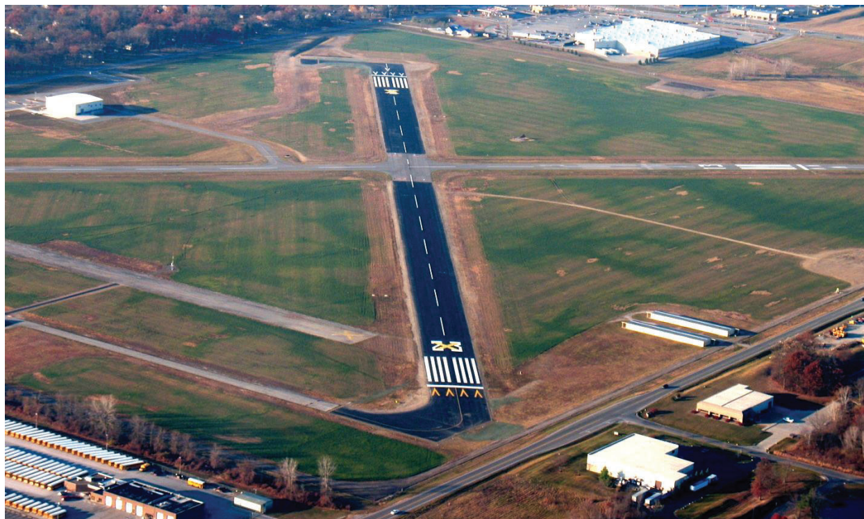
Figure 2-3. Markings for a Temporarily Closed Runway
