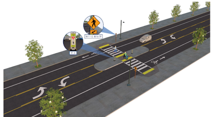
Potential lane configuration for Buckeye Avenue
