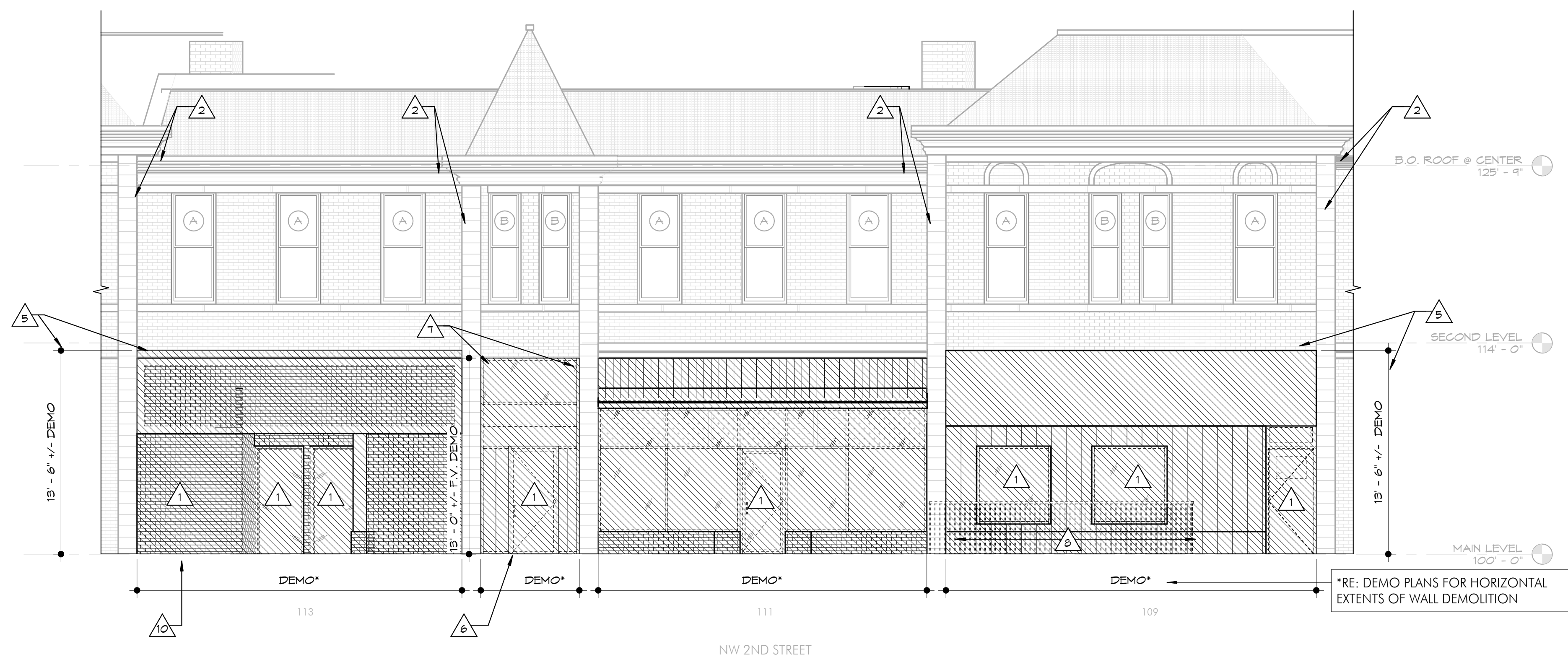
2 south elevation - demolition 3/16" = 1'-0"
