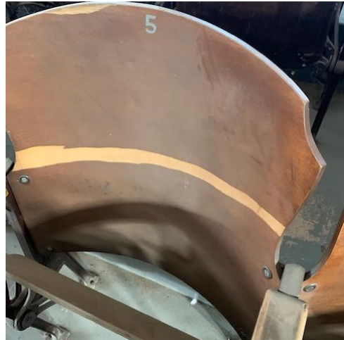
Damaged Wood Veneer
